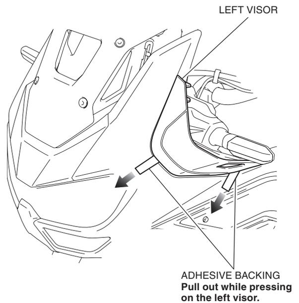
8. Apply adequate pressure to the attached left visor.
